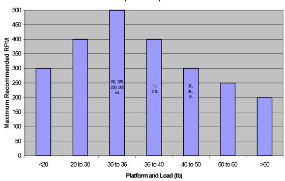
Figure 35: Load & Speed for 1-Inch Orbit Shakers (20% Full)
