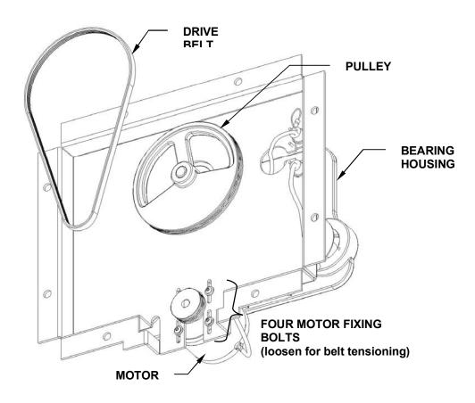
Figure 31: Belt Replacement & Adjustment
