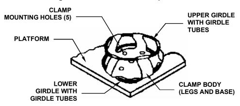
Figure 6a: Clamp Fastener
