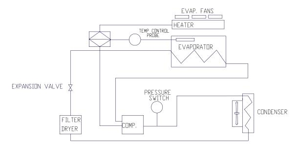
Figure 34: Refrigeration Schematic
