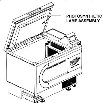
Figure 11: Photosynthetic Lamps (optional)
