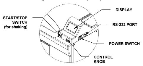
• **START/STOP SWITCH** This switch is used to start or stop the shaker. It will also
